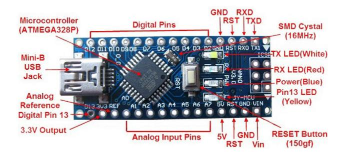
The Nano can be powered via the Mini-B USB connection, 6-20V unregulated external power supply (pin 30), or 5V regulated external power supply (pin 27). The power source is automatically selected to the highest voltage source.
