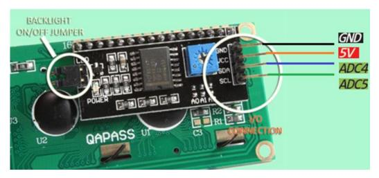
LCD display to Arduino wiring.
